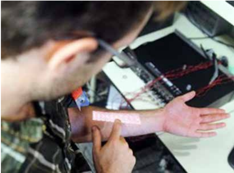
Figure 7. Skinput interface. Chris Harrison, Microsoft Research and Carnegie Mellon Photo Credit: Chris Harrison.
